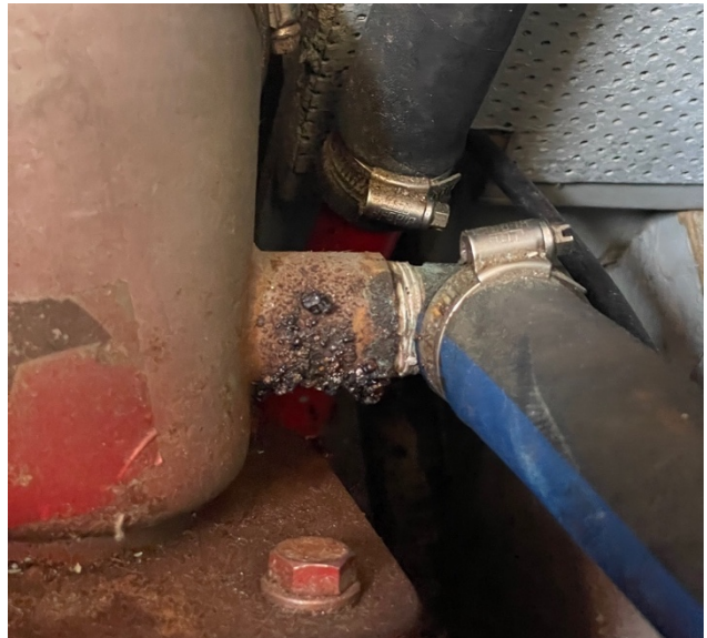
IMG_3511 – Main Engine Exhaust Elbow Corrosion
