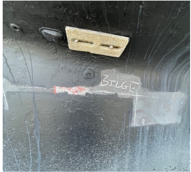
IMG_2517 – Starboard keel side, area of concern outlined in chalk, bilge area marked, damaged transducer and plate zinc.
