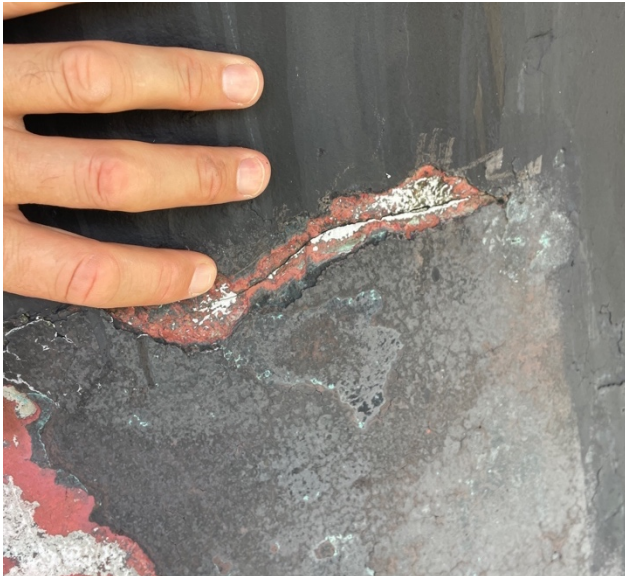
IMG_2516 – Crack at top of fairing, starboard side.
